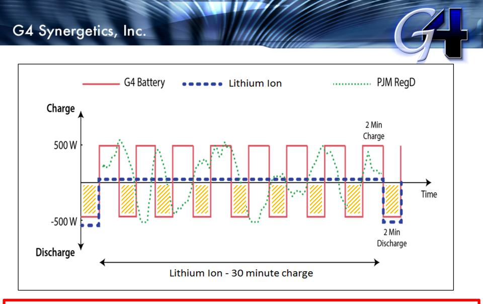
In this model, the G4 Advanced NiMH delivers ~7 times more energy than competitive Lithium-Ion polymer batteries (LPB) at nearly the same power per discharge
