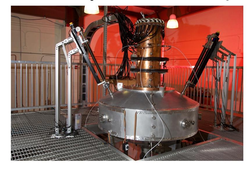
A spheromak is a toroidal confinement plasma where the magnetic fields are produced by currents flowing in the plasma and the toroidal field disappears at the wall.
