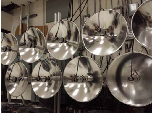
Figure 1- ESC solar simulator
