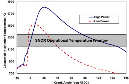
Source: Willand J., Teigeler, M., Wirbeleit, F., Enderle, C., Raab, A., Bockhorn, H., and Schmitt, F., "Selective Non-Catalytic NOx-Reduction in Diesel Engines Using Aqueous Urea," SAE paper 982651, 1998.
