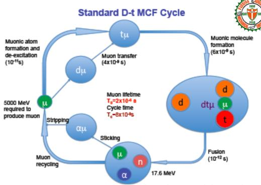
250 fusions are possible in the lifetime of the muon with this cycle time. 3125 fusions per muon are required to break even. 150 fusions have been produced experimentally.
