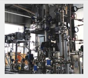
Water-ethanol mixture is sent to proprietary downstream processing equipment separates and concentrates it up to fuel grade ethanol.
