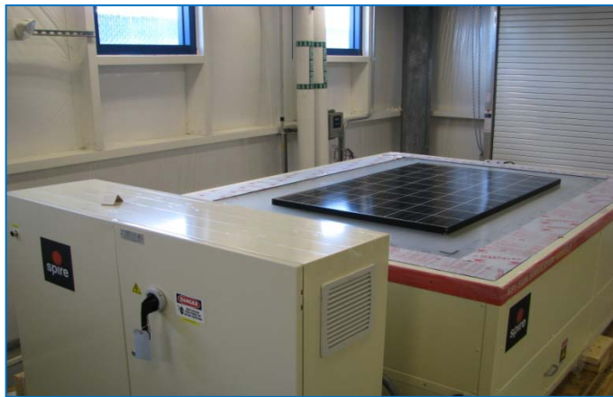
Figure 1. Long-pulse solar simulator for PV module testing
