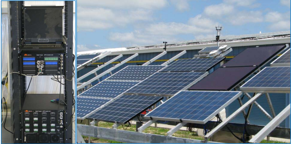
Figure 2. Multi-channel I-V curve tracer (left) capable of continuous testing of multiple PV modules
