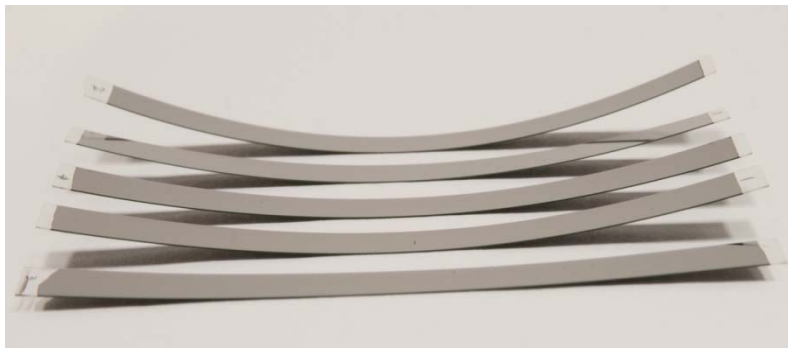
Figure 6. Bending of glass strips at various sputtering conditions.
