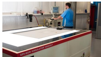
Figure 1: PV module testing with flash simulator
