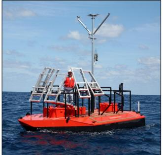
**Figure 5**: Mooring and Telemetry Buoy (MTB) During Open-Ocean Sea Trials.
