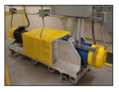
20kw Dynamometer for Generator Testing
