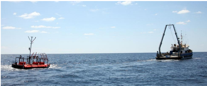
The MTB was towed by the M/V Thunderforce with a drop weight to simulate its moored behavior.
