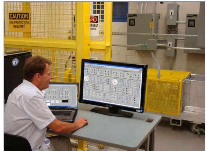
Figure 4: SNMREC dynamometer for generator testing. Unit on left (much of which is hidden by the computer display in the right-hand photograph) is ~3 m long.
