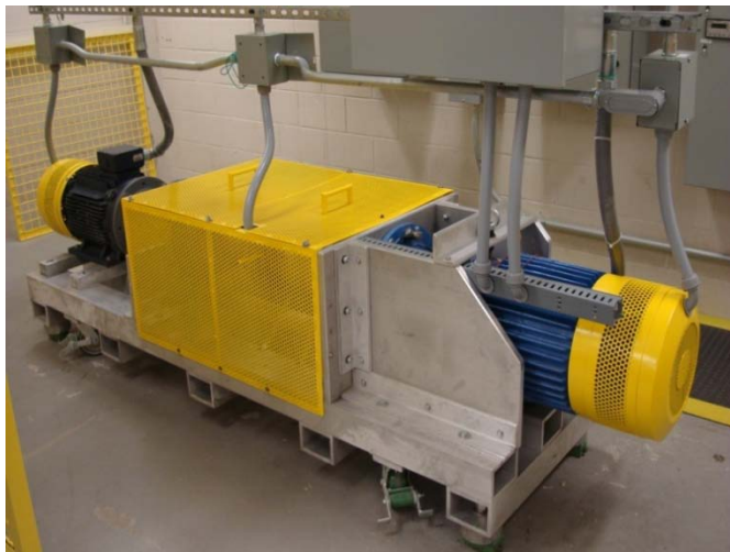
Figure 4: SNMREC dynamometer for generator testing. Unit on left (much of which is hidden by the computer display in the right-hand photograph) is ~3 m long.
