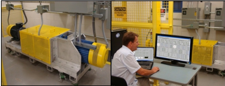
Figure 8. Dynamometer for generator testing (left) and full-up data acquisition and control system (right)
