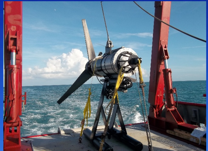
3-meter diameter Rotor, 20kW Instantaneous Max Power Prototype Turbine - At sea after successful deployment 20
