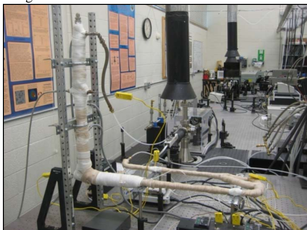
Figure 8: Image of the laboratory-scale reactor used to measure oxidation reaction kinetics under hydrogen production conditions. The capillary for on-line mass spectrometry is visible to the left.
