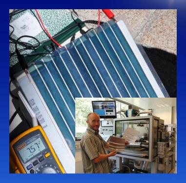
14"x14" polymer solar modules have been printed. 12 cells are connected.
