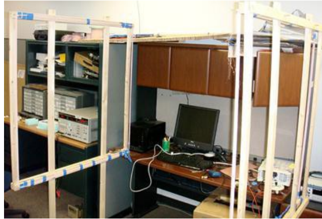
Figure 4: The first wireless power system achieving 38.3 W with 76% efficiency. The coils are made of litz wire: 6 turns, 1 m each side, 1725 strand, 48 AWG.
