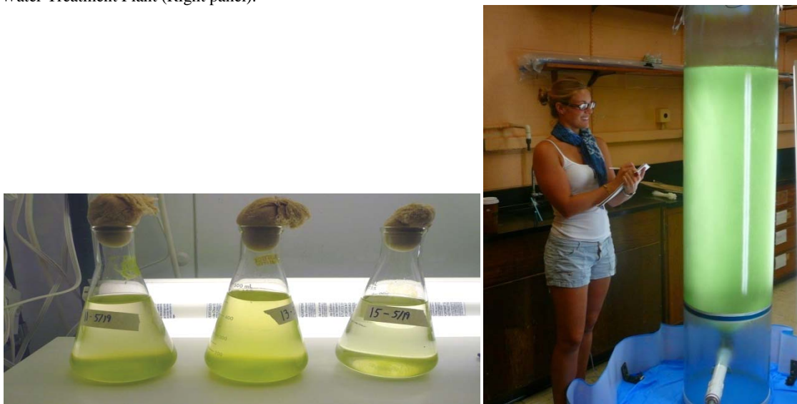
Figure 3. Accumulated microalgal biomass in wastewater (Left panel) and an example of a lab-based bioreactor that we are using for larger-scale microalgal biomass production (Right panel).
