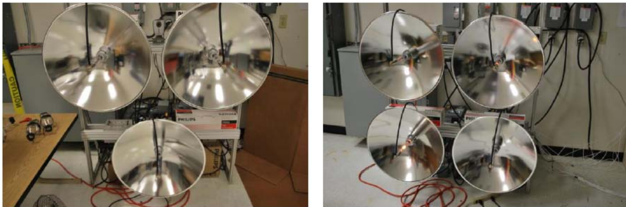
FIGURE 1. LAMP ARRAYS. (left) 3-lamp (right) 4-lamp
