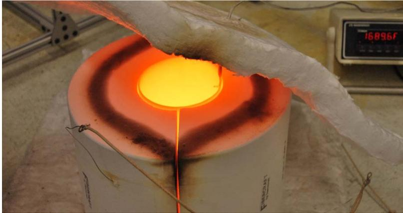
Figure 6: Successful electric heater test reaching core temperature of 1690 F.
