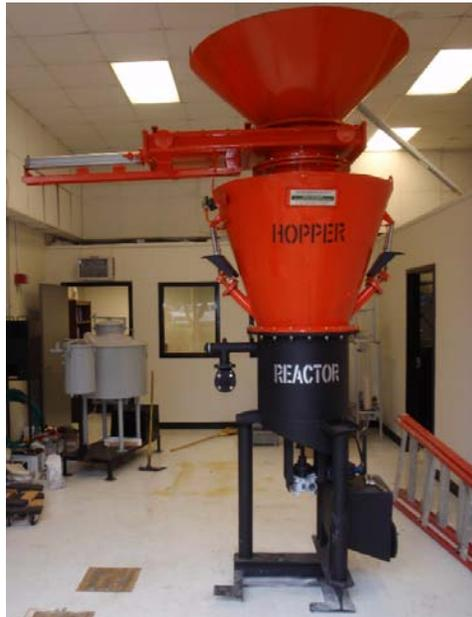
Figure 5: 10 kW commercial downdraft.
