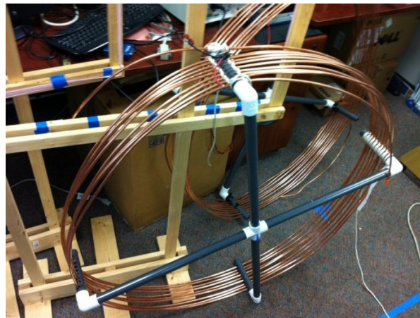
Figure 5: The second wireless power system achieving 114 W and 65% efficiency. The coils are made of ¼” copper tubing on PVC form: 9 turns, 1 m diameter.
