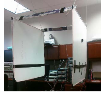
Fig. 1: Wireless electric energy delivery system diagram and picture of test setup (coils are wound around the white cardboards separated by 1 m).
