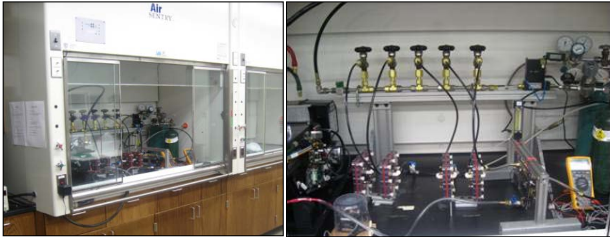
• Instrumented PEM fuel cell station. 1.2 kW stack and single cells
