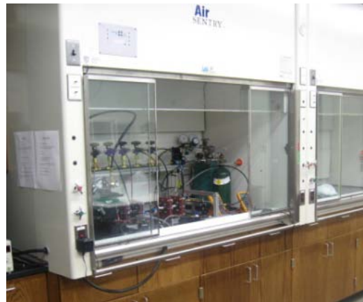
Fig. 1 Instrumental PEM fuel cell station. 1.2 KW
