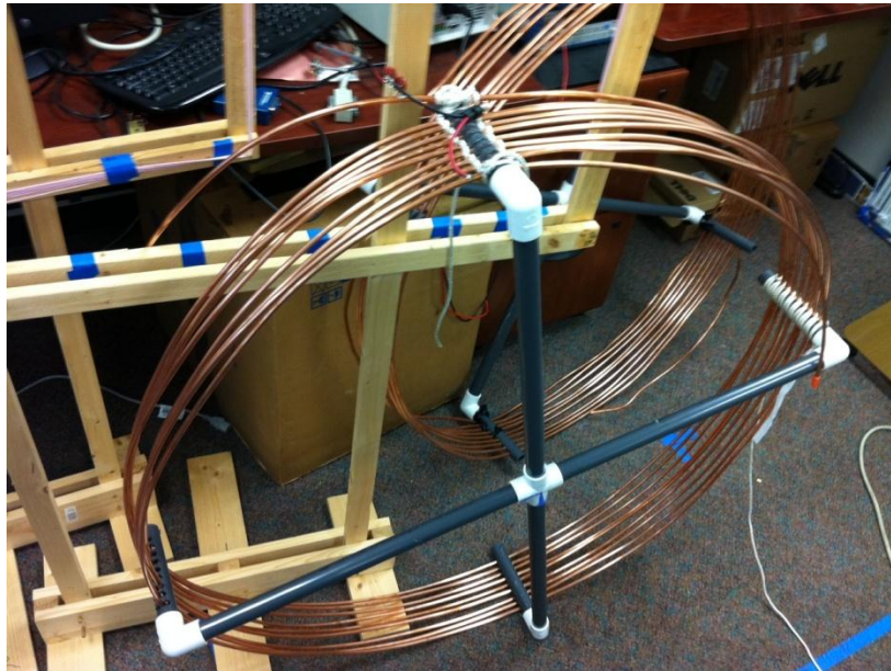
Figure 3: The second wireless power system achieving 114 W and 65% efficiency. The coils are made of 1/4" copper tubing on PVC form: 9 turns, 1 m diameter.
