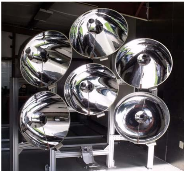
Figure 11 The partially assembled solar simulator at UF.
