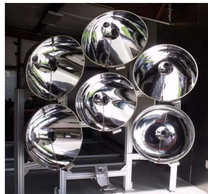
Partially assembled solar simulator
