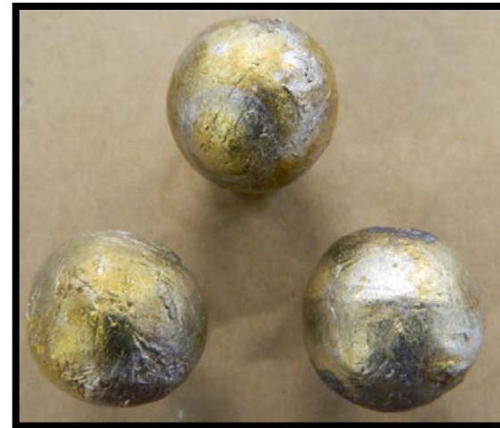
Metalized Capsules to 450°C after 2000 Cycles (6 yrs eqv.)
