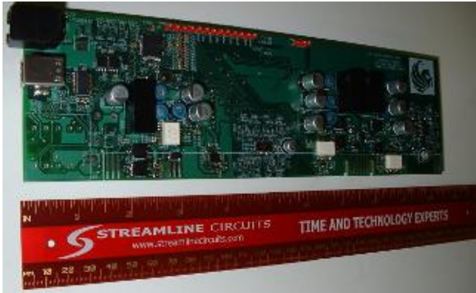
(Above) Controller, MOSFET driving and sensing circuit board
