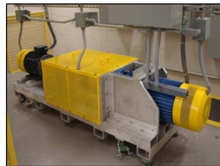
20kw Dynamometer for Generator Testing
