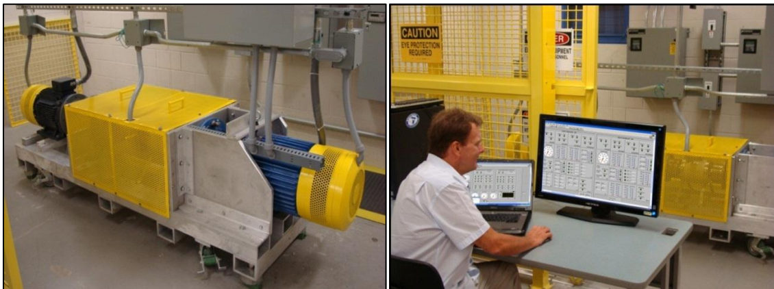
Figure 6: The SNMREC’s dynamometer for generator testing. Unit on left (much of which is hidden by the computer display in the right-hand photograph) is ~3 m long.
