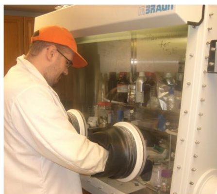
Nick Vito constructing a battery in the Glove Box at UF
