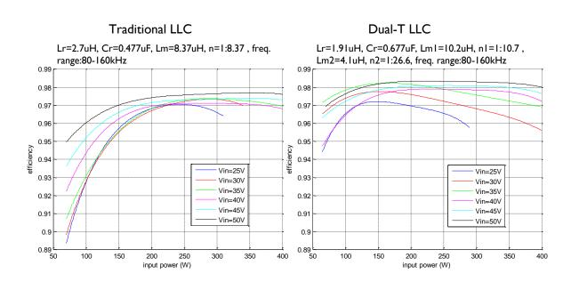
LLC optimal design is to find the circuit parameters that minimize the power loss while maintaining a desired DC gain level to adapt the wide input range. An optimal design procedure is developed based on the mode model. The experiments validate our LLC model study and show promising results of the dual-T LLC topology. A power loss model will be built to further improve the converter efficiency. We will finalize the circuit for its implementation in the mico-inverter prototype
