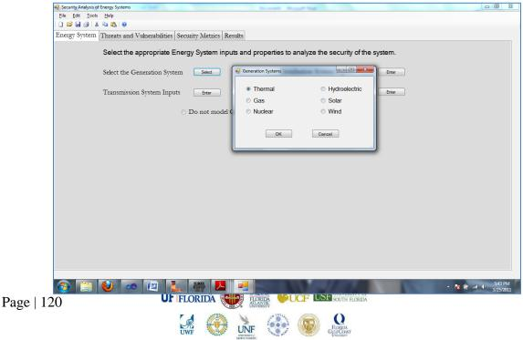
By clicking the Select button, the user can select the type of generation system. This would give the user the ability to analyze the selected energy system. The database at the back-end would contain the elements which are contained in the generation system. Similarly, the user can select the transmission, distribution and control system elements. The inputs are reflected back for the user to review and make changes if needed.
