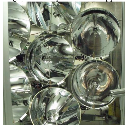
Figure 1a. UF's High Flux Solar Simulator.
