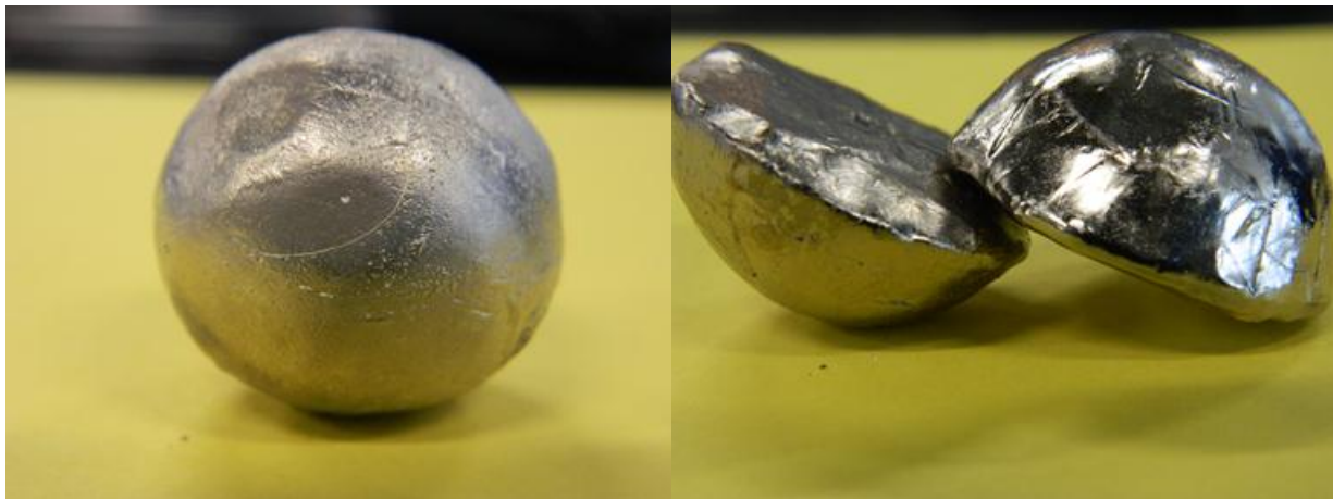
Fig. 8 Metal encapsulated PCM for medium temperature thermal energy storage
