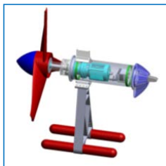
FIGURE 2. SNMREC 3-METER DIA ROTOR, 20KW INSTANTANEOUS MAX POWER PROTOTYPE TURBINE
