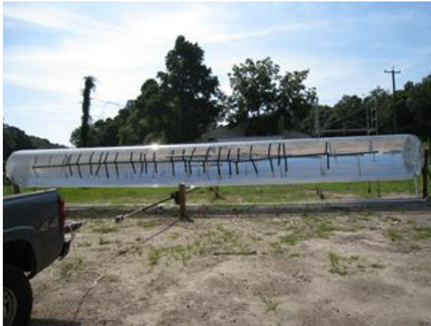
LOAD-ADHESION TESTING OF A 50-FOOT BALLOON
