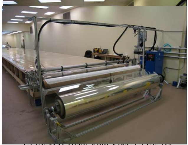
GLUE MACHINE APPLYING GLUE TO THE SOLAR SAUSAGE FORMING AND GLUE MACHINE
