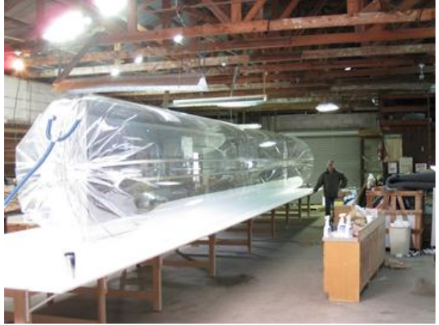
First full-sized inflatable mirror
