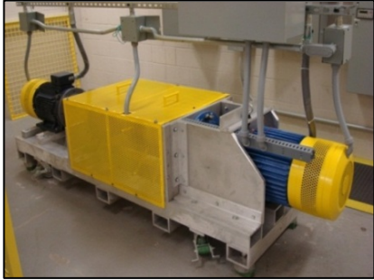
20kW dynamometer for generator testing
