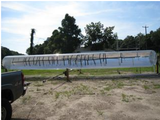
Load-adhesion testing of a 50-foot balloon
