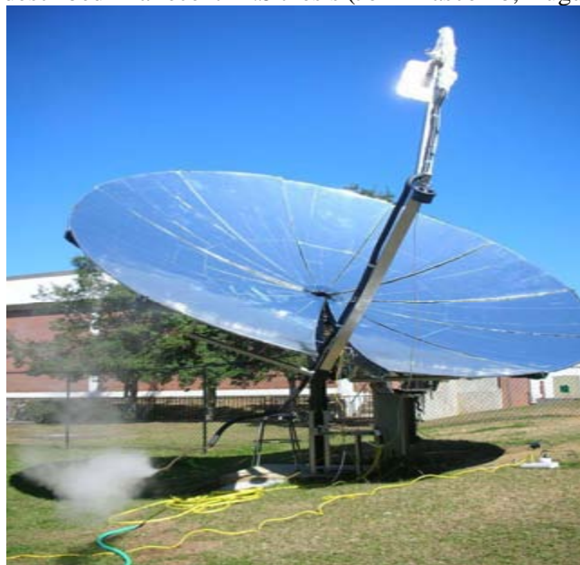
Figure 5. ESC 14 m 2 parabolic dish concentrator with a steam boiler - solar steam generator.
