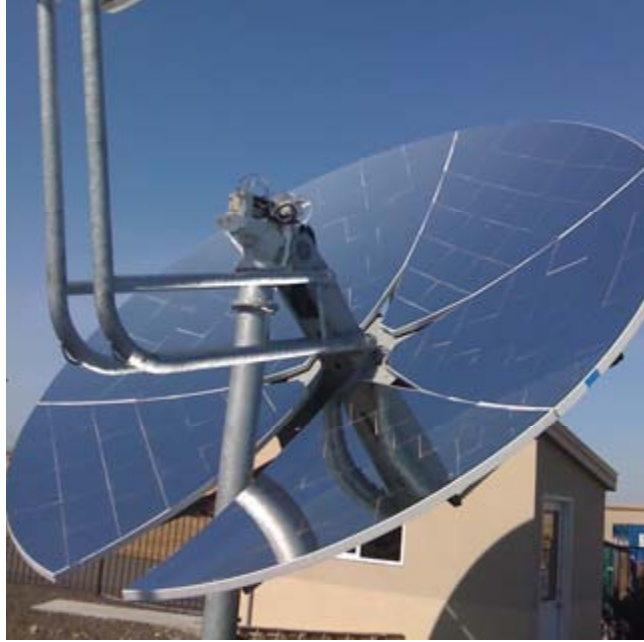
Figure 6. Infinia 3 kW dish-Stirling system.(The dish is being donated to ESC for the steam generation project)
