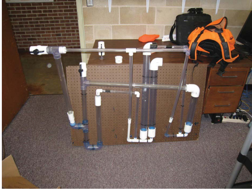
Solenoid type bubbler under construction. The junction in the second column (from left) acts as a solenoid valve. It is flooded with hydraulic fluid to close.
