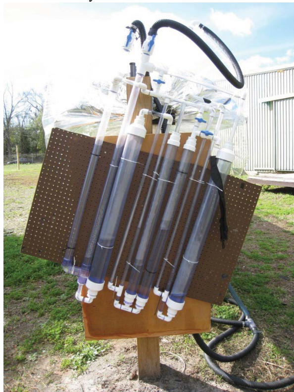
The 10-column "amplifying" bubbler. Again with solenoid action in column 2.
