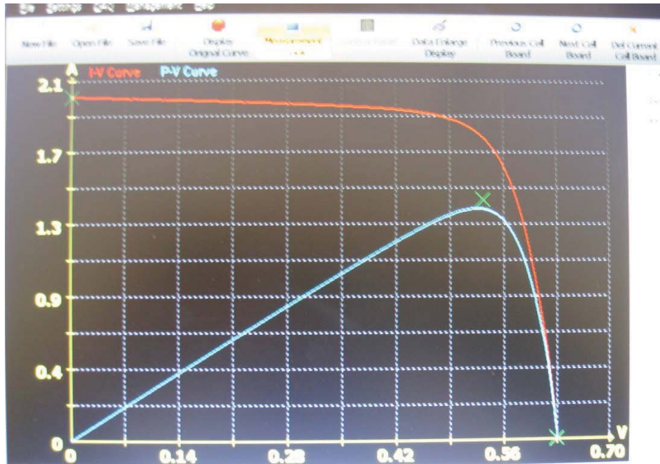
Current-voltage and power-voltage curves of a typical PV cell under 1000 watt per meter square radiation intensity.
