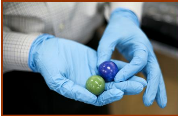
Fig. 7 Ceramic encapsulated PCM for high temperature thermal energy storage
