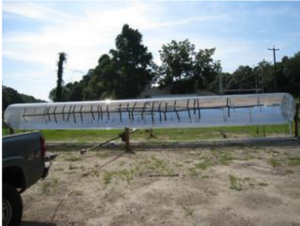
LOAD-ADHESION TESTING OF A 50-FOOT BALLOON
