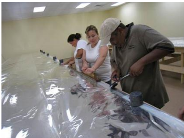
REHEATING THE GLUE TO BOND THE MEMBRANES TOGETHER
