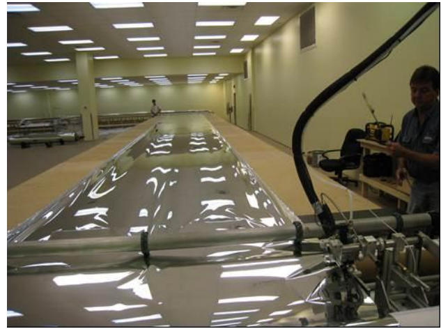
GLUE MACHINE APPLYING GLUE TO REFLECTIVE MEMBRANE
