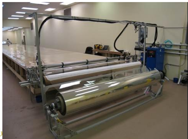
THE SOLAR SAUSAGE FORMING AND GLUE MACHINE
