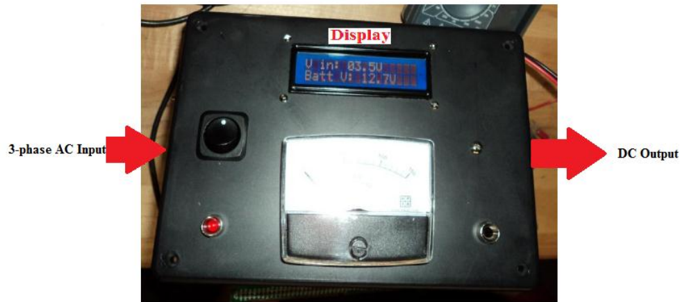
Fig 4. AC-DC converter and battery charging system
