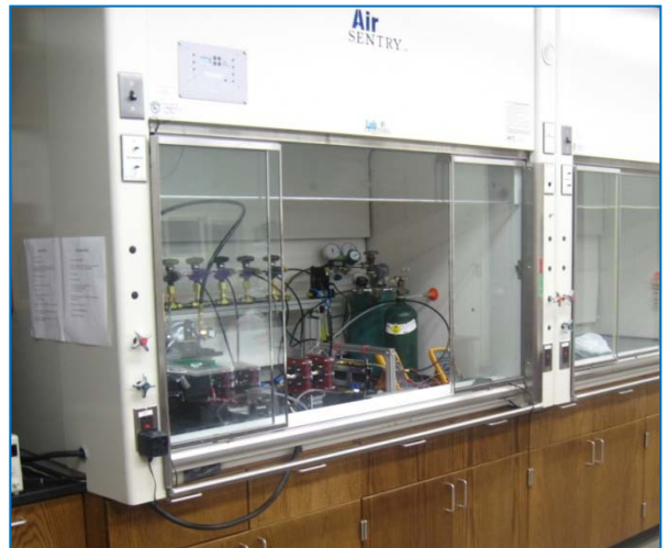
Fig. 1 Instrumented PEM fuel cell station. 1.2 kW.
