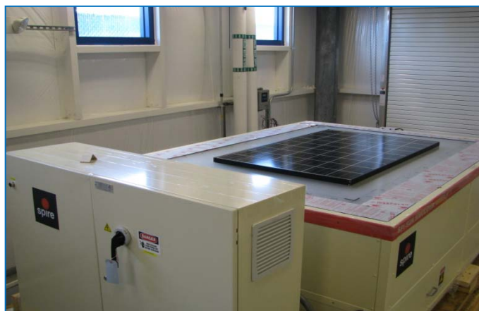
Figure 1. Long-pulse solar simulator for PV module testing
