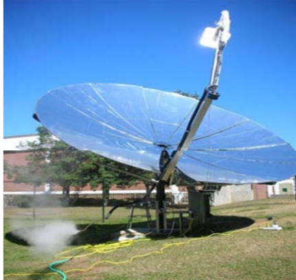
Figure 3. ESC 14 m 2 parabolic dish concentrator with a steam boiler - solar steam generator.
