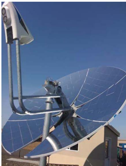
Figure 4. Infinia 3 kW dish-Stirling system. (The dish is being donated to ESC for the steam generation project)
