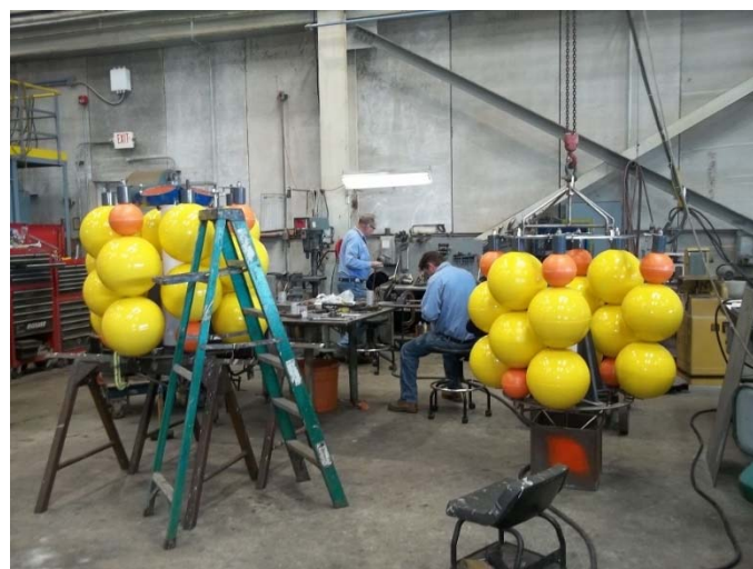
Figure 1 - New ADCP buoys in fabrication.
