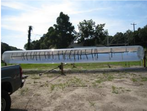
Load-adhesion testing of a 50-foot balloon
