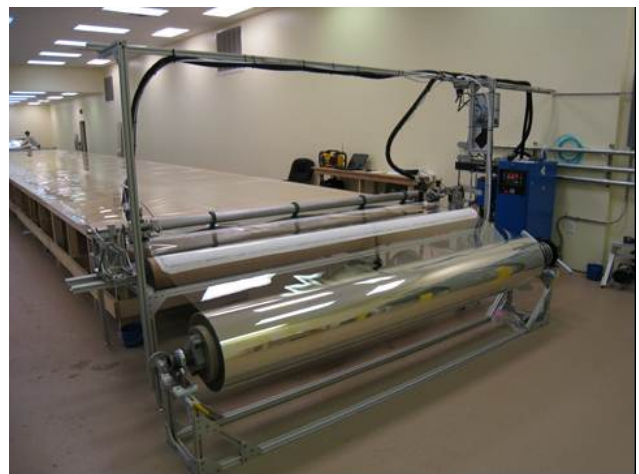
The Solar Sausage Forming and Glue Machine
