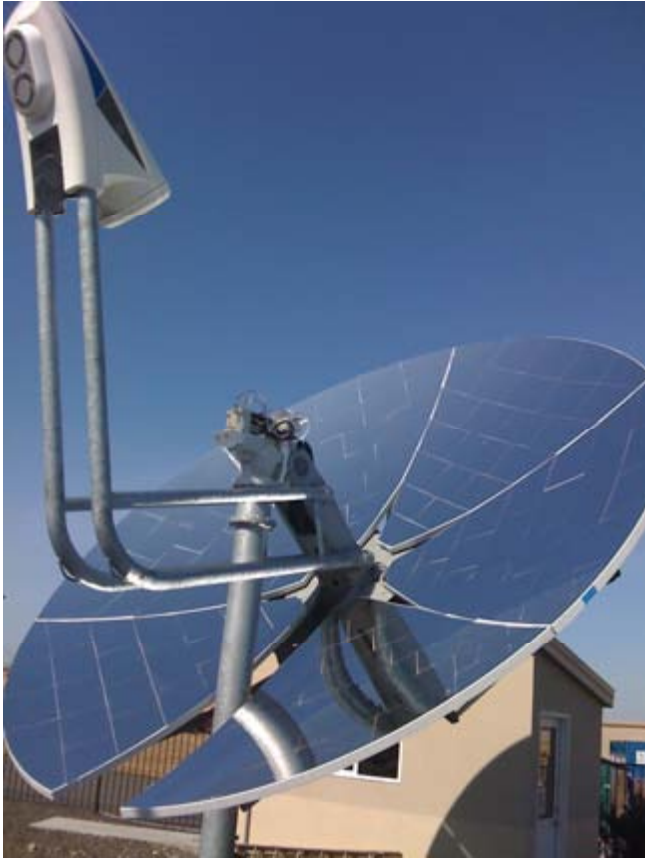
Figure 6. Infinia 3 kW dish-Stirling system.(The dish is being donated to ESC for the steam generation project)
