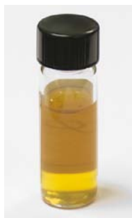
Figure 6. Liquid hydrocarbon product obtained by the F-T synthesis in the presence of combined Fe+Ni/Mo/alumina catalyst.
