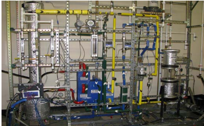
Figure 5 Experimental Setup of the Goswami Cycle
