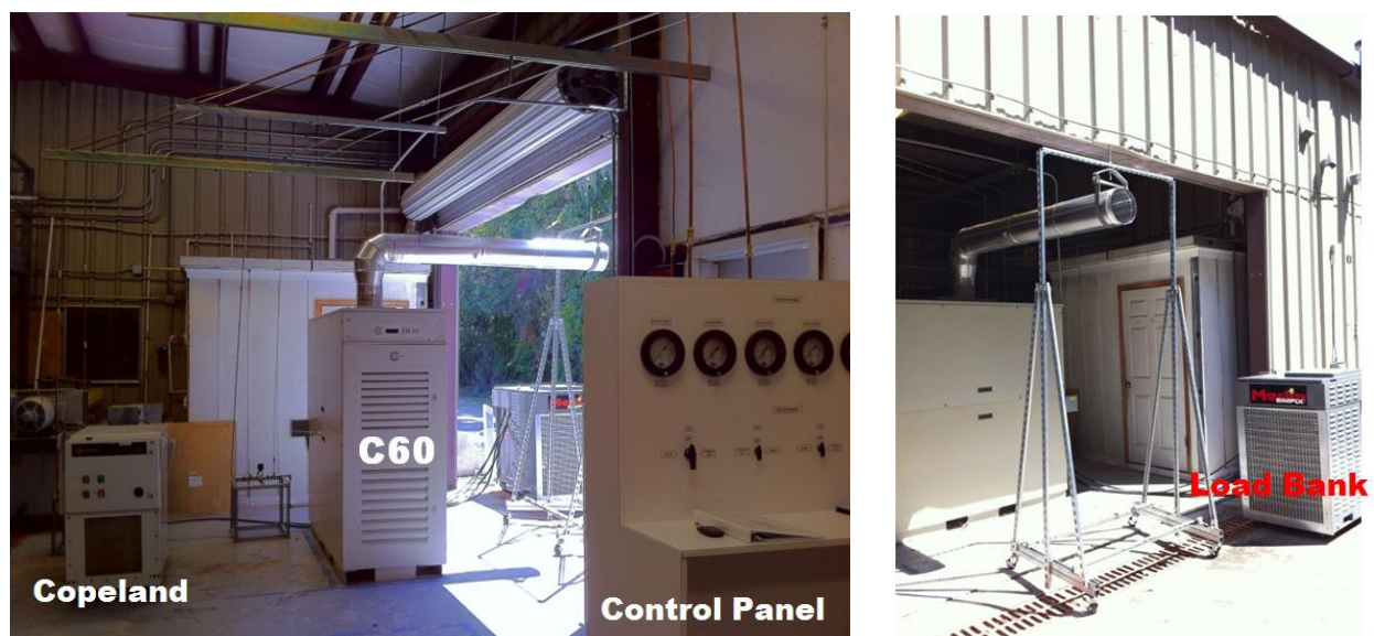
Figure 7: Micro-turbine test system
