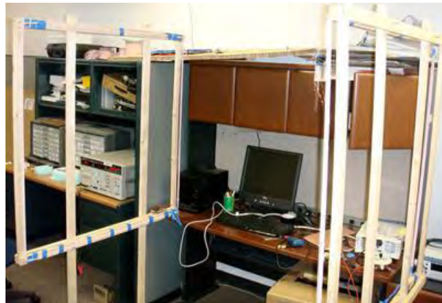
Figure 2: The first wireless power system achieving 38.3W with 76% efficiency. The coils are made of litz wire: 6 turns, 1 m each side, 1725 strand, 48 AWG.
