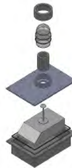
Figure 4b Solar thermogravimeter design, exploded view.
