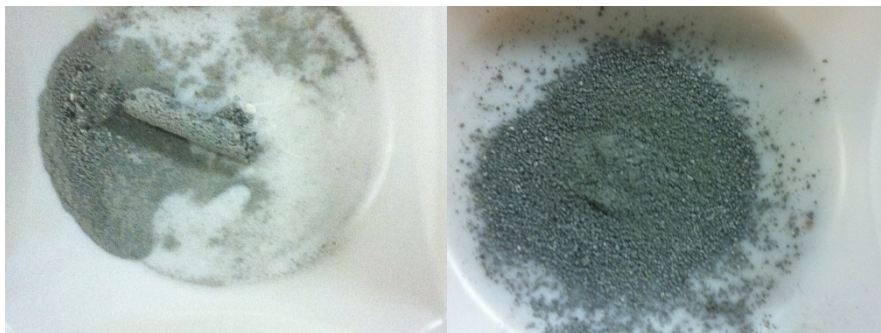
Figure 3: Spent catalyst after 10 cycles. Left: 10wt% Fe precipitated onto n-ZrO 2 and Right: 20wt% iron precipitated onto n-ZrO 2 .
